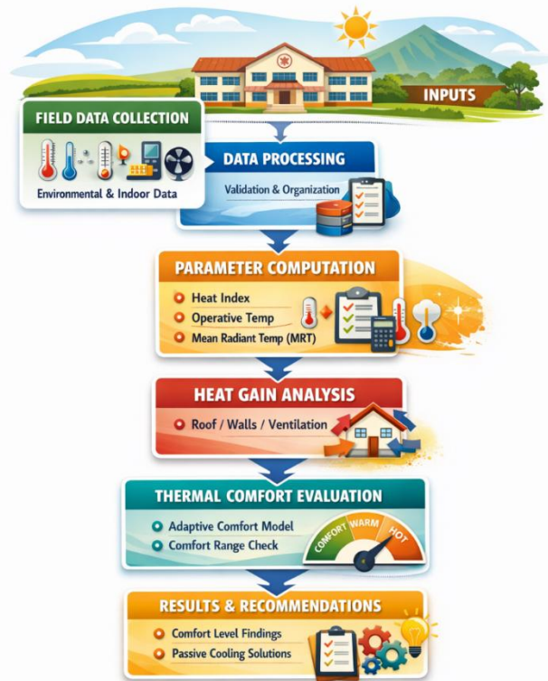
Figure 2. Overview of the naturally ventilated building thermal assessment.
