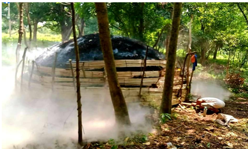
Figure 3: Charcoal production using binulkan method.
