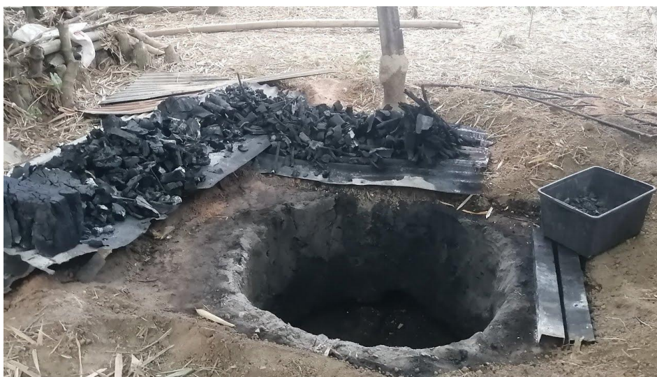
Figure 4: The de bobida dug pit kiln ( pugon )
